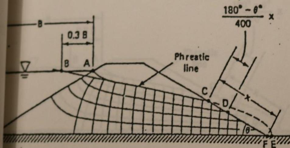
Figure 6.27. Seepage flow net through a homogeneous earth dam. (A portion of the phreatic line  $AD$  can be approximated by the parabola with  $F$  as focus and passing through the point  $B$ . Point  $A$  on the stream face of the dam is the intersection of the water surface with the dam. Point  $D$  is the downstream transition where the seepage is exposed to atmosphere.)
