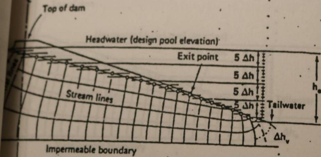
Figure A.1. Gravity affected water table.
