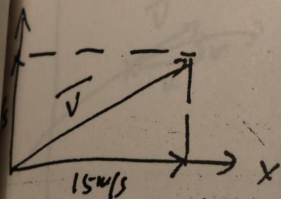
$$\begin{aligned} u &= 5y \\ &= 5(3) = 15 \text{ m/s} \\ v &= 3x \\ &= 3(2) = 6 \text{ m/s} \end{aligned}$$
