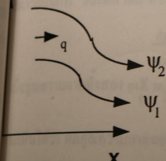
$$q = \int_{\Psi_1}^{\Psi_2} d\Psi = \Psi_2 - \Psi_1 \quad \dots\dots\dots(4)$$
