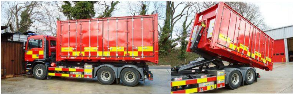
Photo 2 Multilift hook-lift loading system
