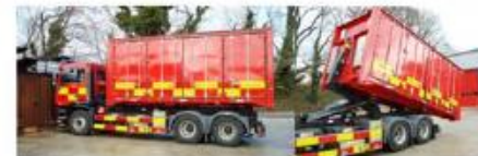
Photo 2 Multilift hook-lift loading system
