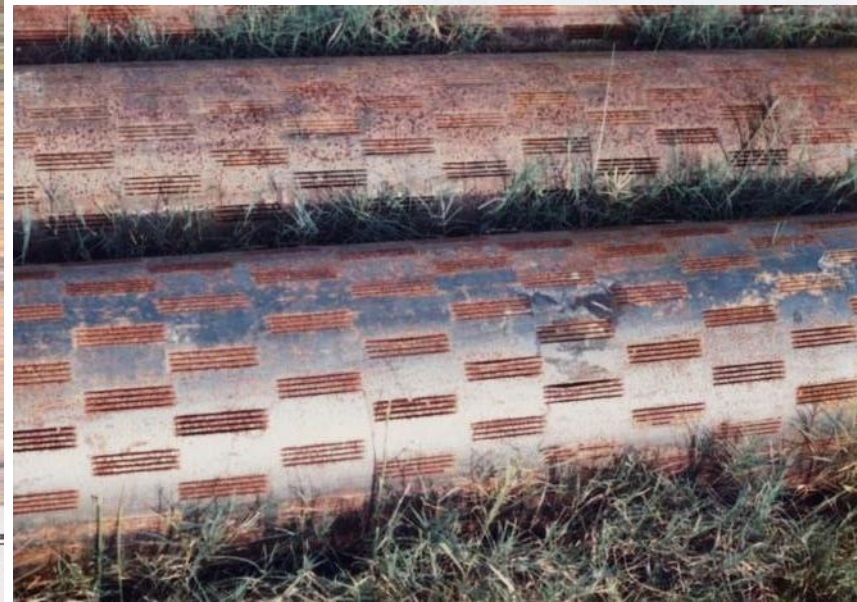
Figure 12.10. A pipe-base screen is constructed by wrapping wire around, or placing a continuous slot screen over, a perforated pipe base. This exceptionally strong construction is often specified for oil wells and occasionally for deep water wells. Both steel and plastic materials are used in this type of construction.
