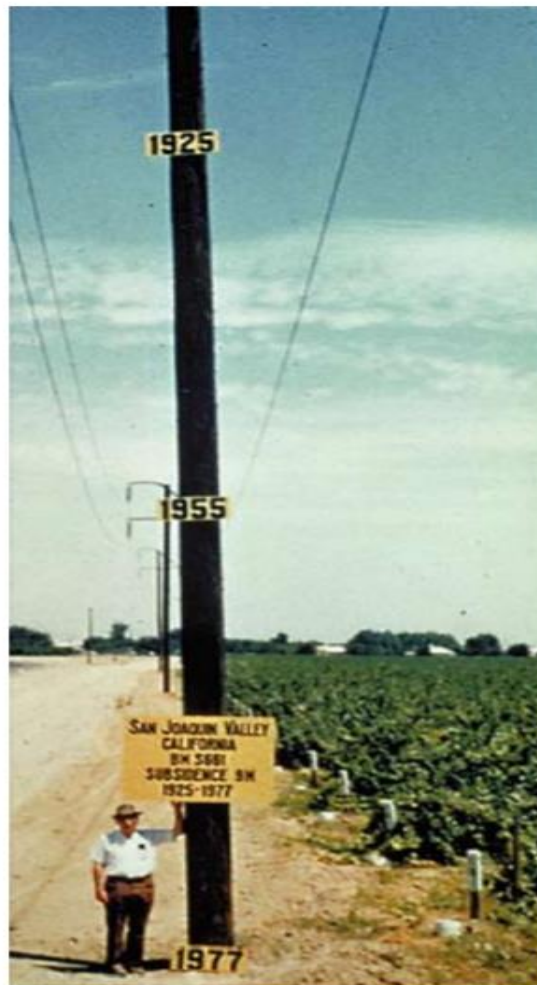
Figure 22. Land subsidence in the San Joaquin Valley, 1926-70 (modified from Poland and others 1975). The approximate location of maximum subsidence (28 feet) in the United States is Mendota, San Joaquin Valley, CA. Signs on the pole show approximate altitude of the land surface in 1925, 1955, and 1977 (Galloway and others 1999).
