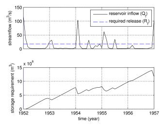
**Figure 2.** Example of sequent peak algorithm: (a) time series of streamflow  $(Q_t)$  and required release  $(R_t)$ , and (b) corresponding storage requirement: the reservoir would be designed based on the maximum value
