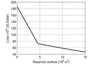
**Figure 3.** Loss for municipal water users as a function of reservoir outflow (for 1 month), based on reference water demand
