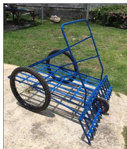
Fig. 2. Wheelbarrow rake set. For canals with a bottom width of 1.0 to 2.0 meters.
