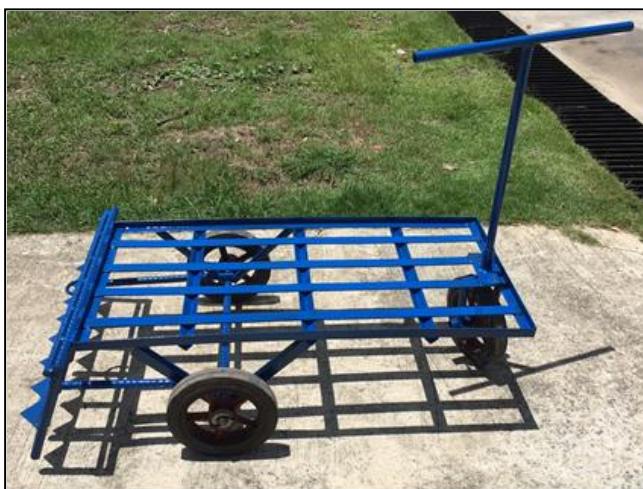
Fig. 1. - Cart rake set. For canals with a bottom width of 0.5 to 1.0 m.
