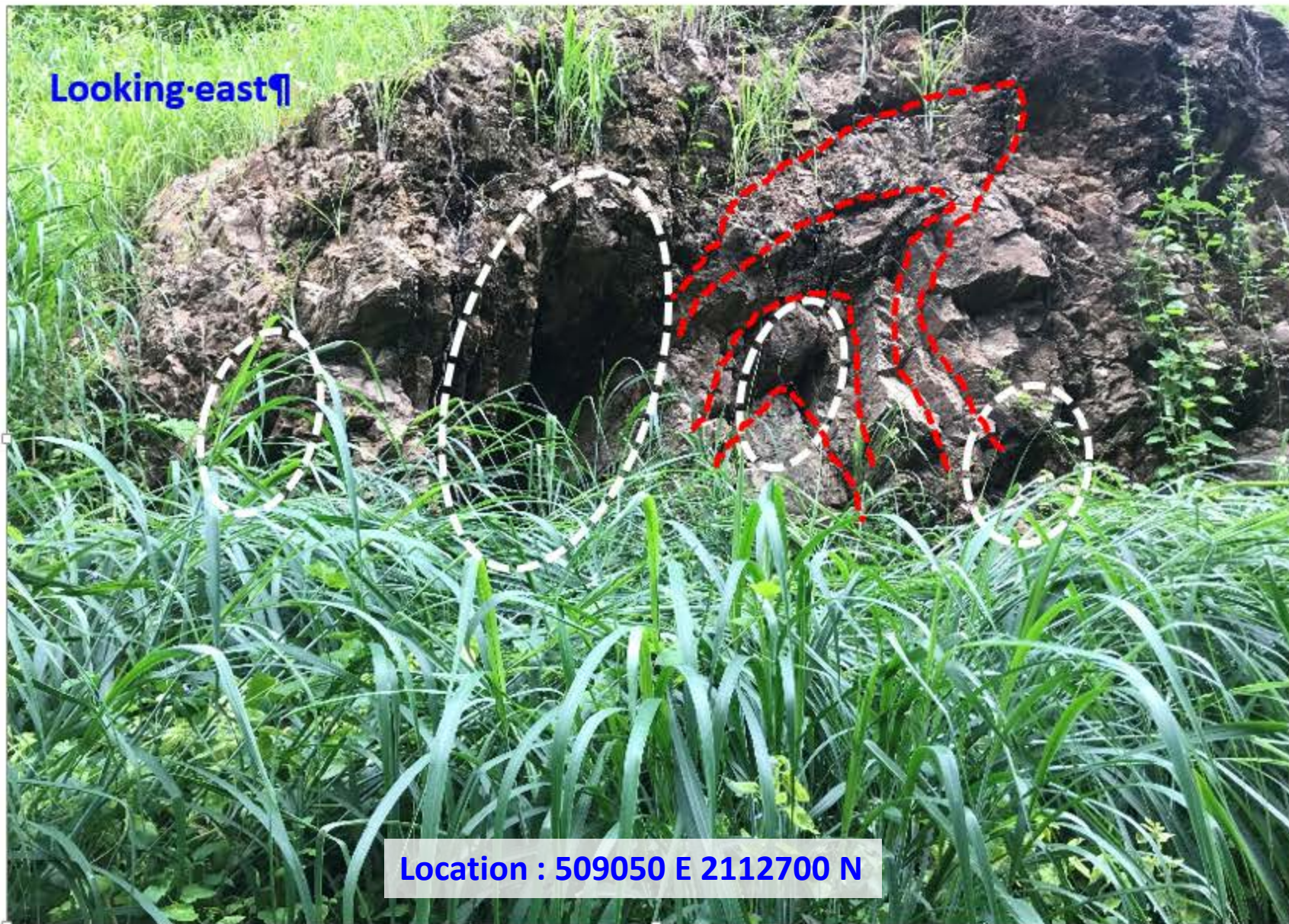
Fig.1. Rock exposures at Huai-Khun-Mi , showing opened joint, fracture, and cavity (white), associated with fold structure (red) as channels that water outflowing from reservoir.
