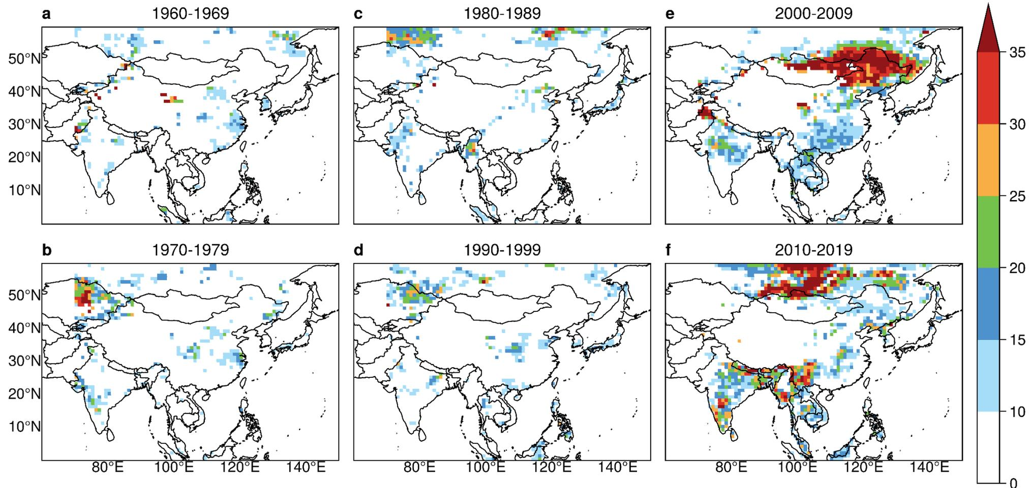
Fig: Number of months under severe soil moisture drought
