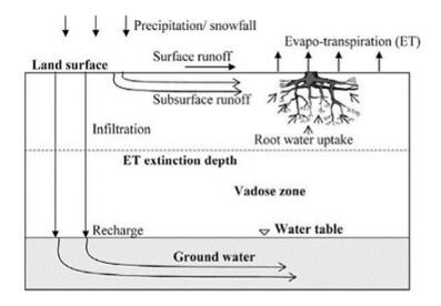
A schematic showing the processes affecting subsurface hydrology (Source: Twarakaviet al., 2008)
